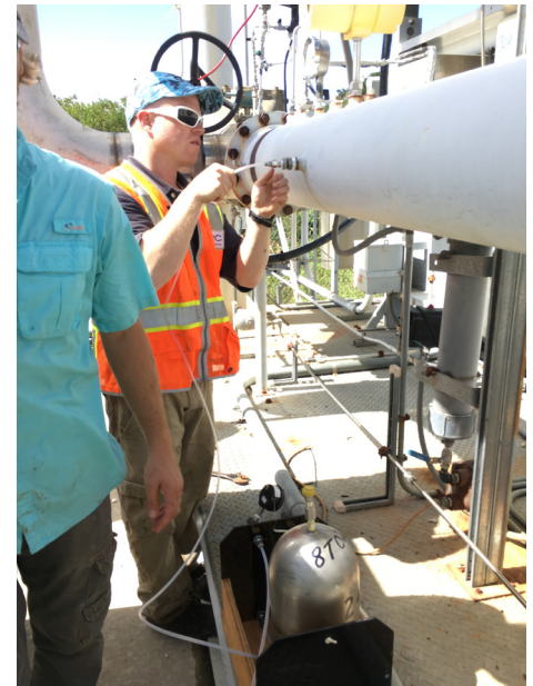
Figure 1 - Sampling of landfill gas from header pipe.
