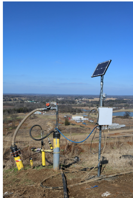
Figure 1 - SCS eTools landfill gas monitoring equipment.
